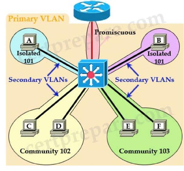
The Private VLAN (PVLAN) Edge feature, also known as protected ports, ensures that there is no exchange of unicast, broadcast, or multicast traffic between protected ports on the switch.
