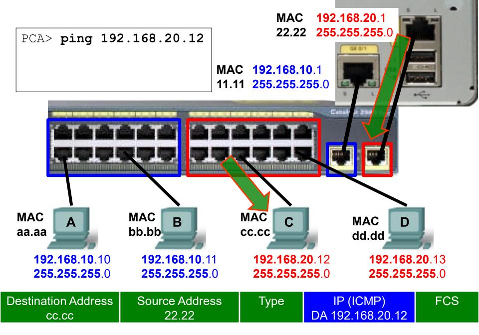
Router sends Ethernet frame to final destination, PC-C
