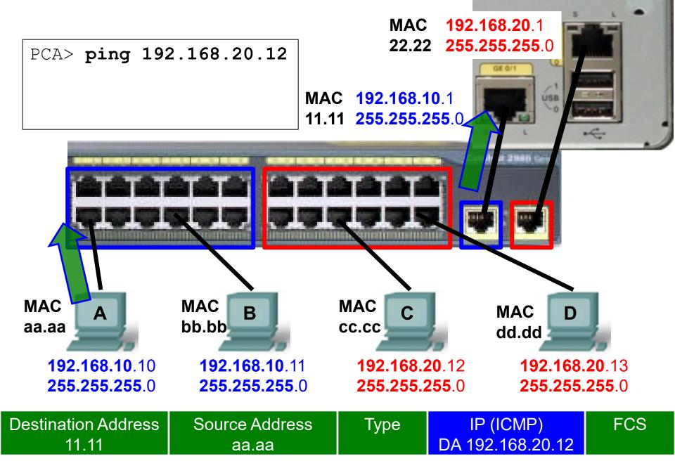
A sends Ethernet frame to default gateway, the router
