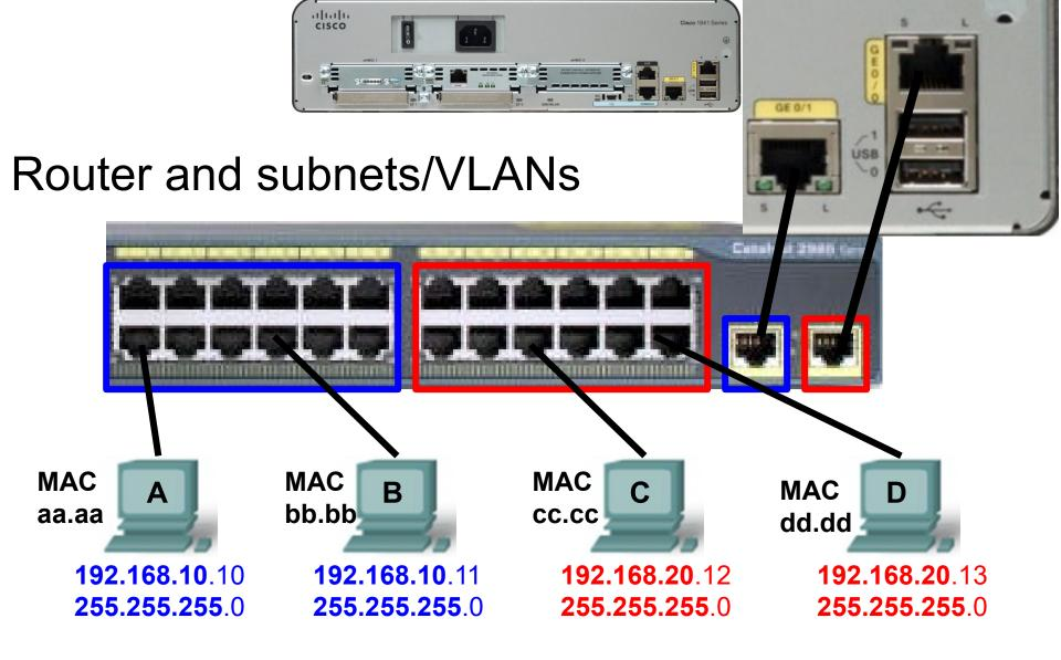
Router is required to connect (route) between subnets/VLANs
