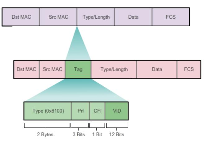
The TAG is added by the switch before it goes over a trunk link.
