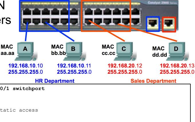
S1# show interface fa 0/1 switchport Name: Fa0/1 Switchport: Enabled Administrative Mode: static access Operational Mode: down Administrative Trunking Encapsulation: dotlg Negotiation of Trunking: Off Access Mode VLAN: 10 (HR) Trunking Native Mode VLAN: 1 (default) Administrative Native VLAN tagging: enabled Voice VLAN: none Operational private-vlan: none Trunking VLANs Enabled: ALL <some output omitted> S1#
